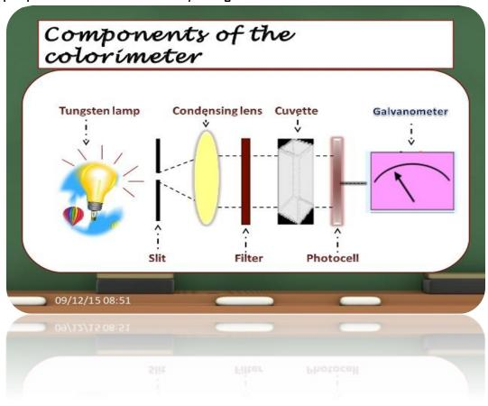
**WORKING SYSTEM OF COLORIMETER-**When using a colorimeter it requires being calibrated first which is done by using standard solution of the known concentration of the solute that has to be determined in the test solution. For this, the standard solution are filled in the cuvette holder in the colorimeter.
