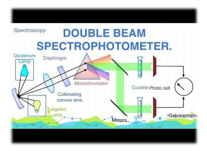
First the source of radiation, it may be UV-light, visible light or infra ray, UV-ight can be obtained by heating the filament with hydrogen. Second is collimator lens and then the monochromator, after monochromator there are two mirror are placed, after mirror there are two cuvette, one for sample and other for blank solution finally the photocell connected to computer from which we get signal.
