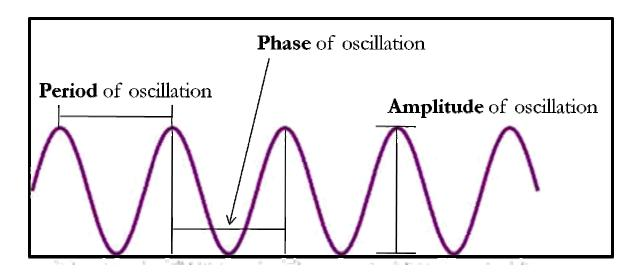
Time required to complete one cycle – **Period**. A particular recognizable point in a cycle – **Phase**. Maximum Displacement of mass from the zero position – **Amplitude**.
