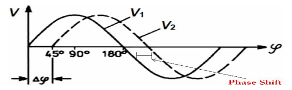
The displacement of the rhythm without altering the basic character of the oscillation is called **Phase Shift**.
